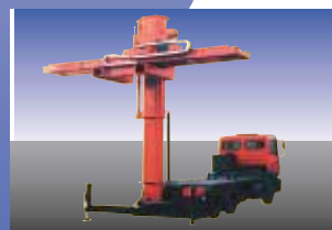
Various transport and handling systems for heat exchangers are available for assisting the cleaning operation.
